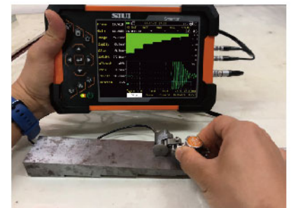
With PES-02D for encoded B-Scan
